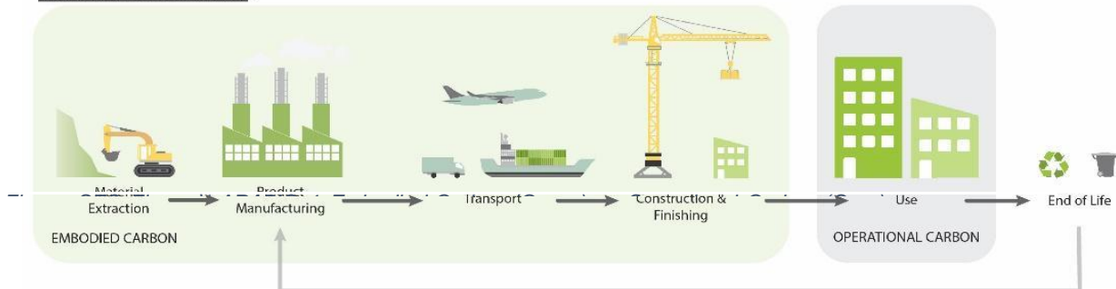
Figure 1. Embodied and operational carbon. Source: Created by AHL and used with permission.
