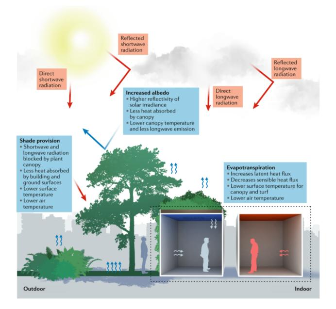
*Greenery-related cooling mechanisms in the urban environment.* Urban greenery acts to modify shade provision, evapotranspiration, and albedo. The combination of these three mechanisms reduces sensible heat gain, thereby, lowering heat gain and surface temperature. Red boxes indicate warming mechanisms and blue boxes indicate cooling mechanisms.
