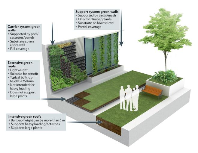
**Types of greenery on buildings.** Different options for vertical and rooftop greenery, including support system green walls, carrier system green walls, extensive green roofs and intensive green roofs.
