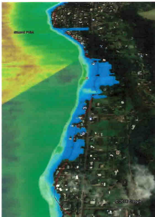
Figure 4. Model result showing the erosion (red line) and annual wave run-up (blue) under 98 cm (3.2 ft) of sea level rise at Sunset Beach, Oahu's North Shore. This is an oblique image of model results found at the Hawai'i SLR Viewer. 50
